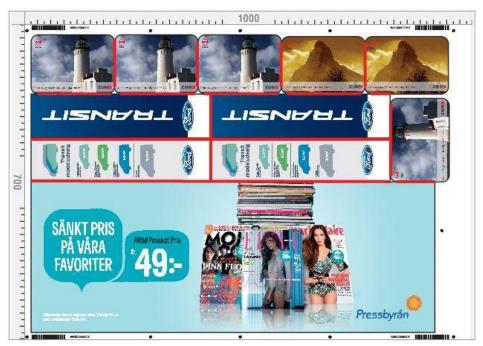
The above red lines indicate which parts of a nesting that could be used for common line cutting.
